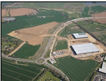
The works involved the excavation, placement and Firmafil treatment of 110,000m<sup>3</sup> of cohesive soils to form the development platform. The works were carried out over the period November 2014 to April 2015. As the site was developed in a flood plain the excavated materials came from a flood compensation area which was formed to a shape as agreed with the Environment Agency before being restored to farmland.
